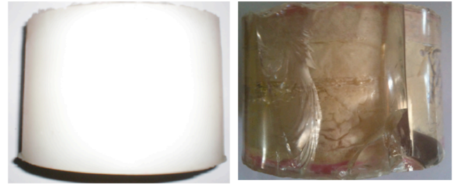
Fig. 9. Results of drop test from 1 m height for silicone rubber (left) and polyester resin (right) samples. The polyester resin has noticeable cracks.
