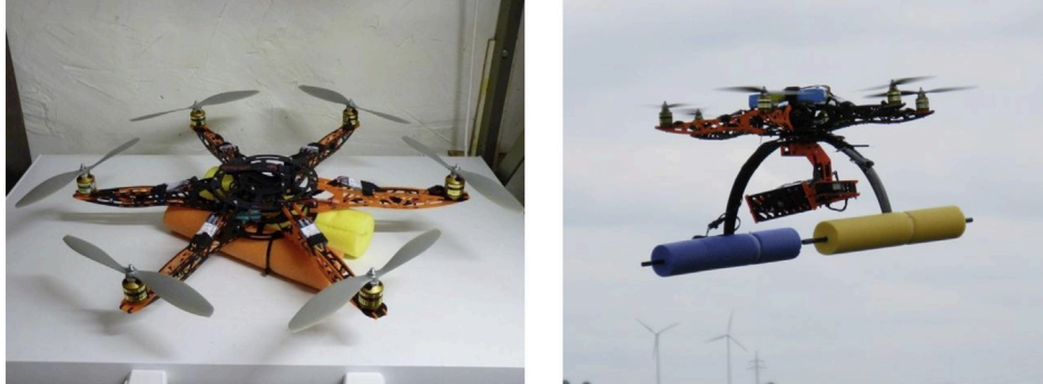
Fig. 3. e Hexacopter used to take low-altitude aerial photographs (Jannoura, R., et al., 2015)
