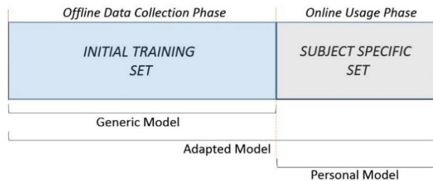
Figure 2. Training sets used for different models: (1) Generic, (2) Adapted, and (3) Personal.
