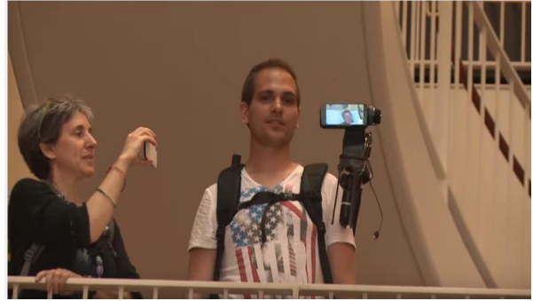
Figure 5: Polly telepresence device. Shoulder worn metaphorical "parrot on shoulder" provides telepresence to remote person.
