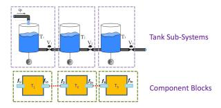
Fig. 3. Diagram of the three-tank system.
