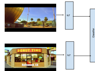
Figure 1: Pairwise comparison based Training: Concatenated images features (fc7) from same trailer are fed to the classifier and it learns to predict the more interesting image
