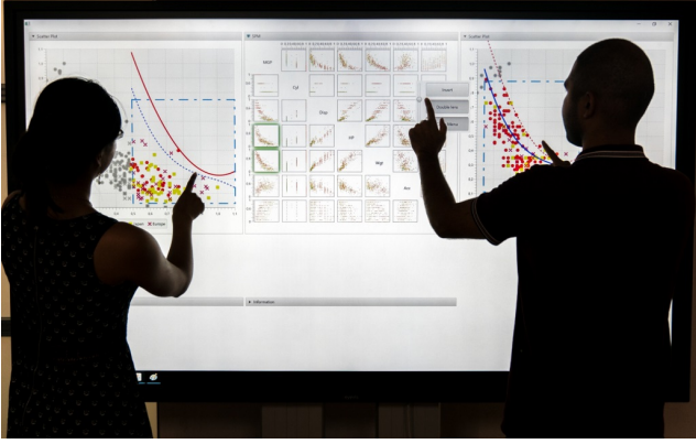
Fig. 1. Two users collaboratively analyse a dataset on a large vertically-mounted multi-touch screen. User A on the left drags a Regression Lens, while user B on the right adapts the degree of the regression model using the floating toolbox. The display is an Eyevis 84-inch 4K/Ultra-HD 60Hz multi-touch LCD monitor with a resolution of 3840 \times 2160 .
