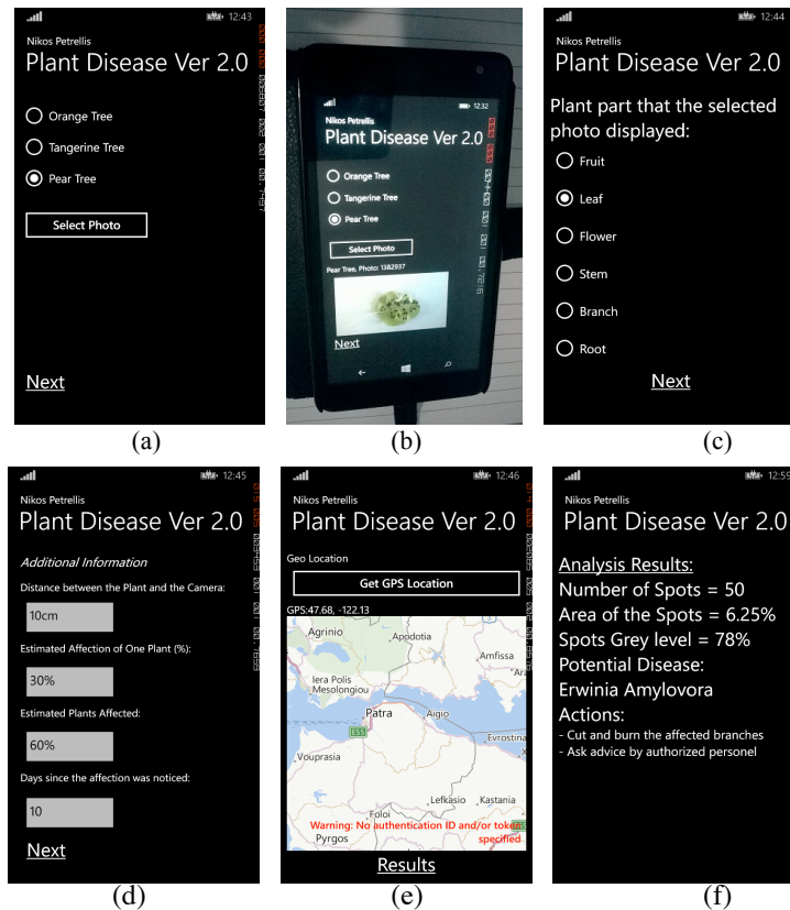
Fig. 3. Pages of the developed application. Initial page (a) and initial page after the photo selection (b). Selection of the plant part the photo displays (c). Additional Information entered by the user (d). Geolocation for retrieving statistical and weather information about the area (e) and the results page (f).
