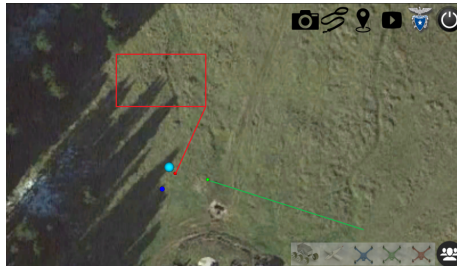
(e) Touch Screen User Interface. In red an area to explore, in green a path to navigate.
