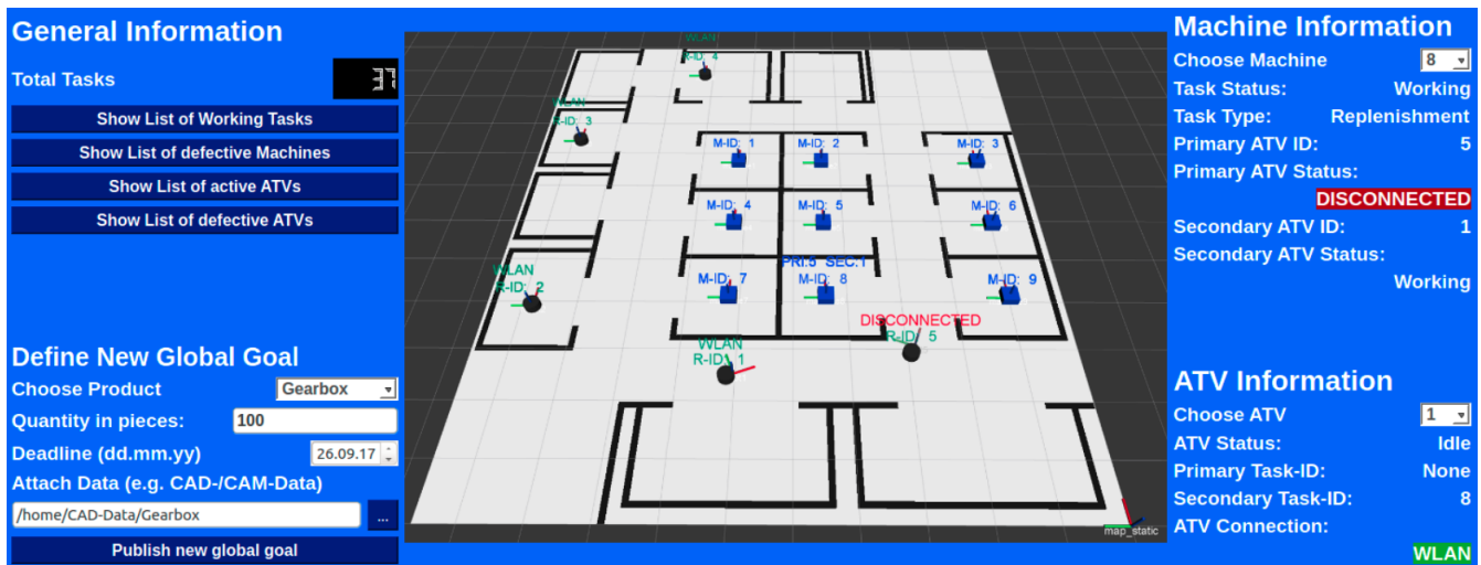
Figure 4: Management Panel is used for surveillance purposes by visualizing the plant in ROS ( center ) and displaying several information about the plant (top left), the machines (top right) and the ATVs (bottom right). Additionally, it is used to define and publish global production targets (bottom left).
