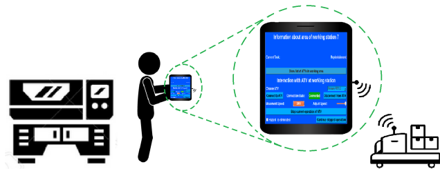
Figure 5: Operator at the machine connects to and interacts with an ATV via handheld device
