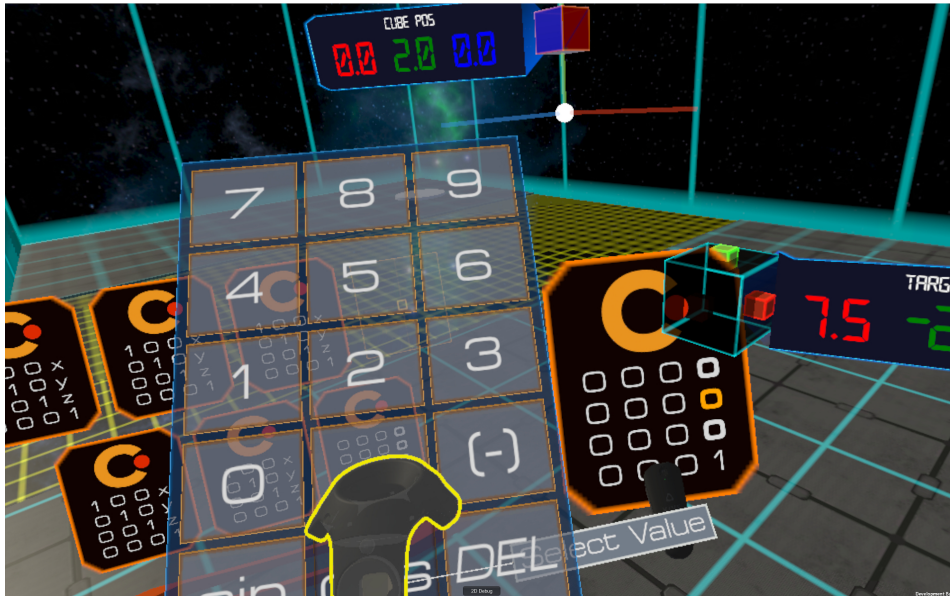
Fig. 8: GEtiT-VR allows for a direct value input via a special input matrix UI.
