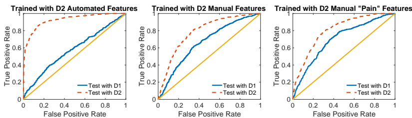
Fig. 2. ROC Curves for classification within and across domains using automated features (left), manual features (middle) and pain-related manual features (right). The red dotted lines are ROCs when the machine is able to use environment information to differentiate pain and no-pain conditions, and the blue solid lines show the machine’s ability to discriminate between pain and no-pain based on AU information alone. The straight yellow line graphs the performance of random chance.
