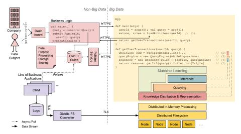
Fig. 1. SPIRIT architecture exemplifying the transparency use case
