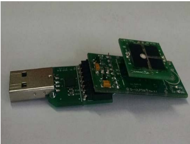
Fig.2. Connected DGS-NO 2 968-037 to USB-Bridge UART
