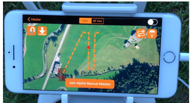
Fig. 3. User interface showing the search path and location for an individual drone. The slanted line in the beginning shows the drone is directed to fly in a direction away from the other drones in the area.
