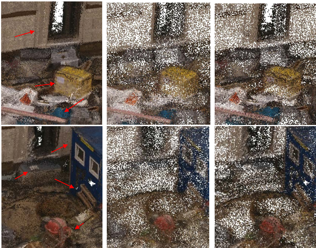
Figure 4 a-f: Dataset “construction site”: (a, d) high-res, (b, e) low-res; (c, f) filtered point cloud. The arrows indicate preserved features. Compared to the low-res reconstruction the filtered cloud shows higher geometric contrast.
