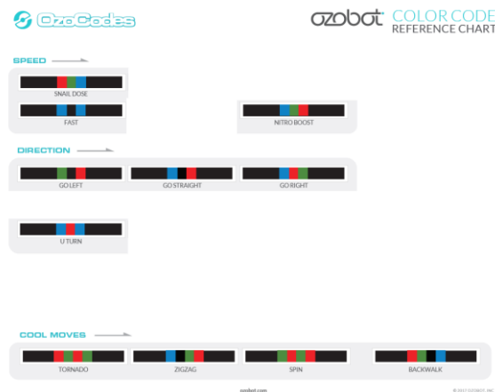
Fig. 3: Ozobot color code reference chart used in the experimental phase
