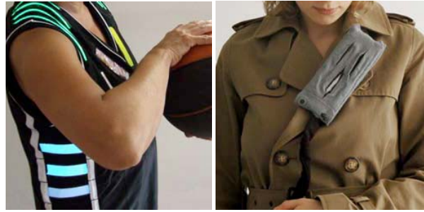
Figure 3. Wearable ambient visualization. Left: a light-emitting basketball jersey showing game-related information (Designer: Mitchell Page, [14]); Right: a wearable folding device conveying activity information (Designer: Monika Hoinkis, [16]).
