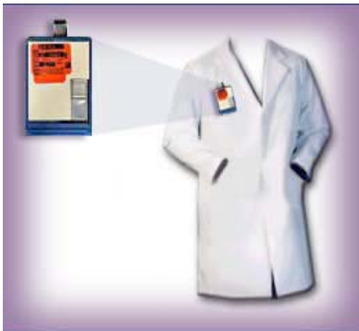
Figure 2: Classical worn dosimeter. The badge changes color based on amount of exposure to radiation
