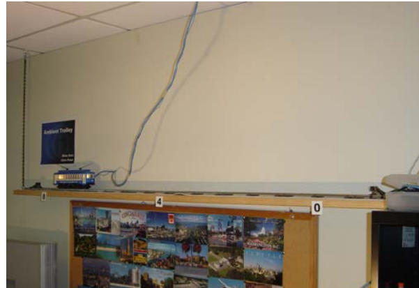
Figure 3: Configuration of Ambient Trolley showing tracks and positional markers used to indicate distance from trolley stop.
