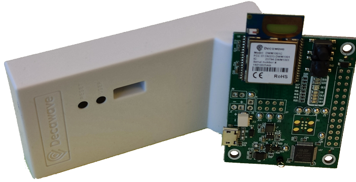
Figure 2: Decawave’s DWM1001 Development Board, which has been utilized in the experiments.
