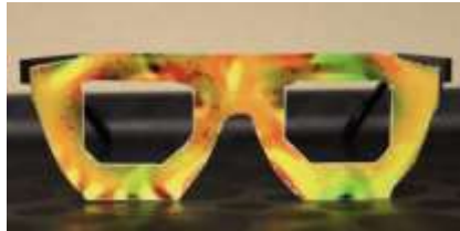
Fig. 4. Example of glasses that can be used to trick the face recognition system
