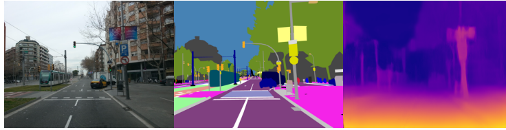
Fig. 1: Sample of the data used when training the perception model. The left image is the original RGB. The center image is segmentation ground truth from Mapillary. The right depth map was generated from RGB images with the Monodepth2 network.
