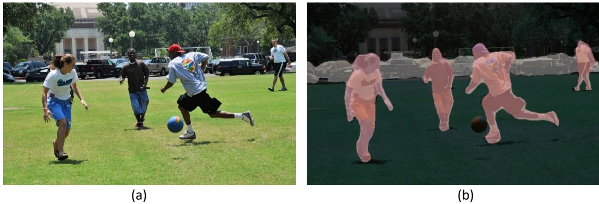
Figure 2: Images: before (a) and after (b) segmentation using the Pixellib library
