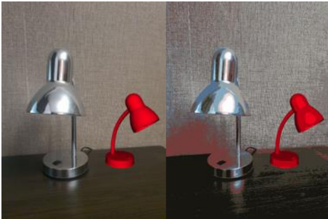
Figure 4: The result of image processing by the K-Means algorithm
