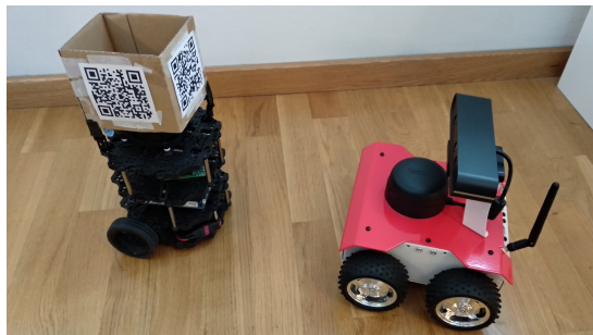
Figure 3: Rosbot 2.0 following a QR code-equipped TurtleBot3.
