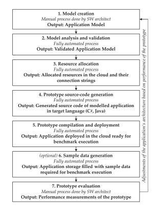
Figure 1: Prototyping process
