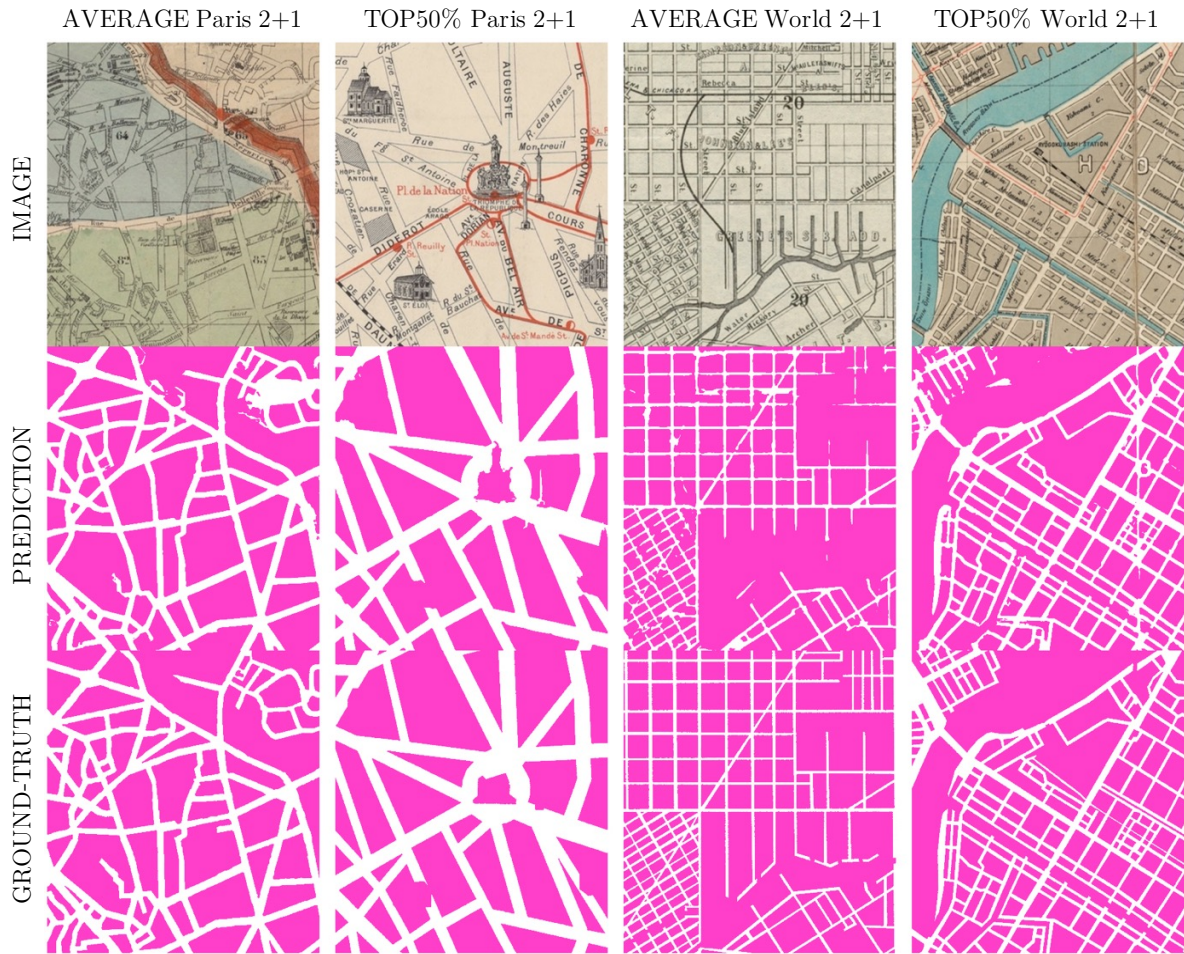
Figure 7: Examples of results. Each time, the first example is close to the median mIoU and the second is part of the top 50%. Values of the mIoU from left to right: 0.8965, 0.9506, 0.8079, and 0.8622.
