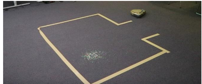
Figure 1: Image of the floor as staged for the user testing. Framed as a playful navigation task, the tape represents walls for the user to navigate the robot around, with the goal of vacuuming all the rice thrown on the floor.
