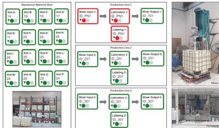
Figure 7: Real-time Monitoring Dashboard showing the Raw Material Warehouse and the Production Lines
