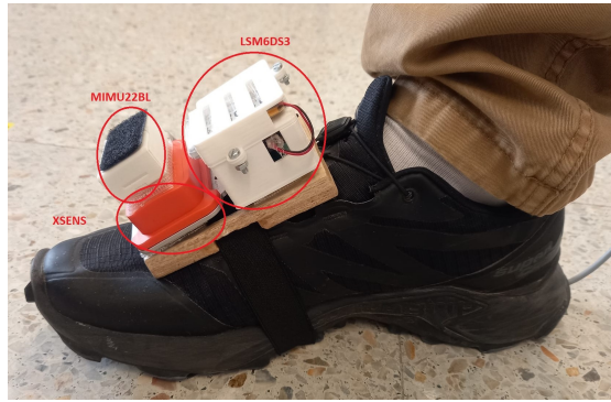
Figure 5: Attachment of the IMUs on the right foot of one test subject.
