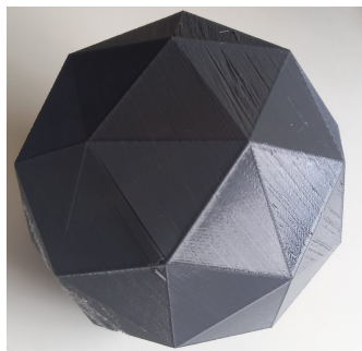
Figure 3: 3D printed pentakis dodecahedron used for the calibration of the different IMUs.
