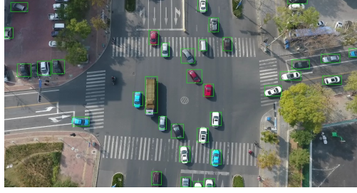
Figure 2: Output of the vehicle detection phase based on a frame from the M0603 scene.
