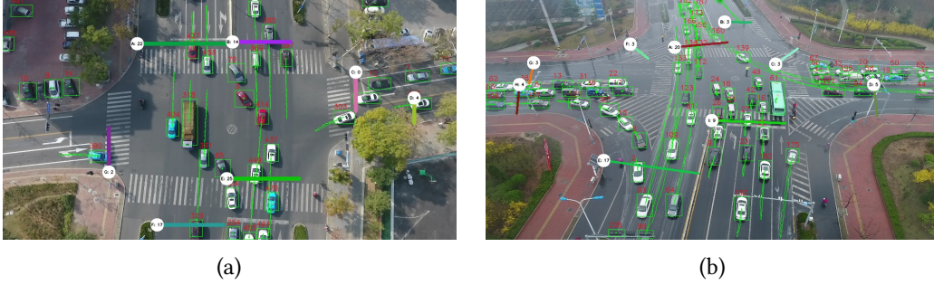
Figure 5: Identification of the origins and destinations of the vehicles based on frames from the M0603 (Fig. 5a) and M0403 (Fig. 5b) scenes.
