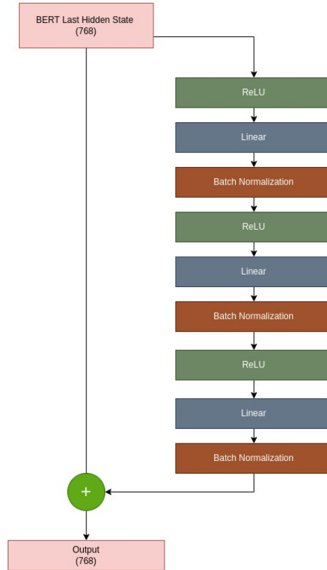
Figure 3: Graphical representation of the residual block module, containing three linear layers with activation function ReLU and batch normalization.
