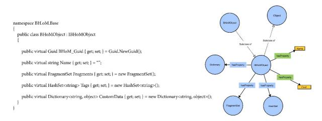
Figure 1: BHoM\_Object base (left) and its corresponding graph (right).
