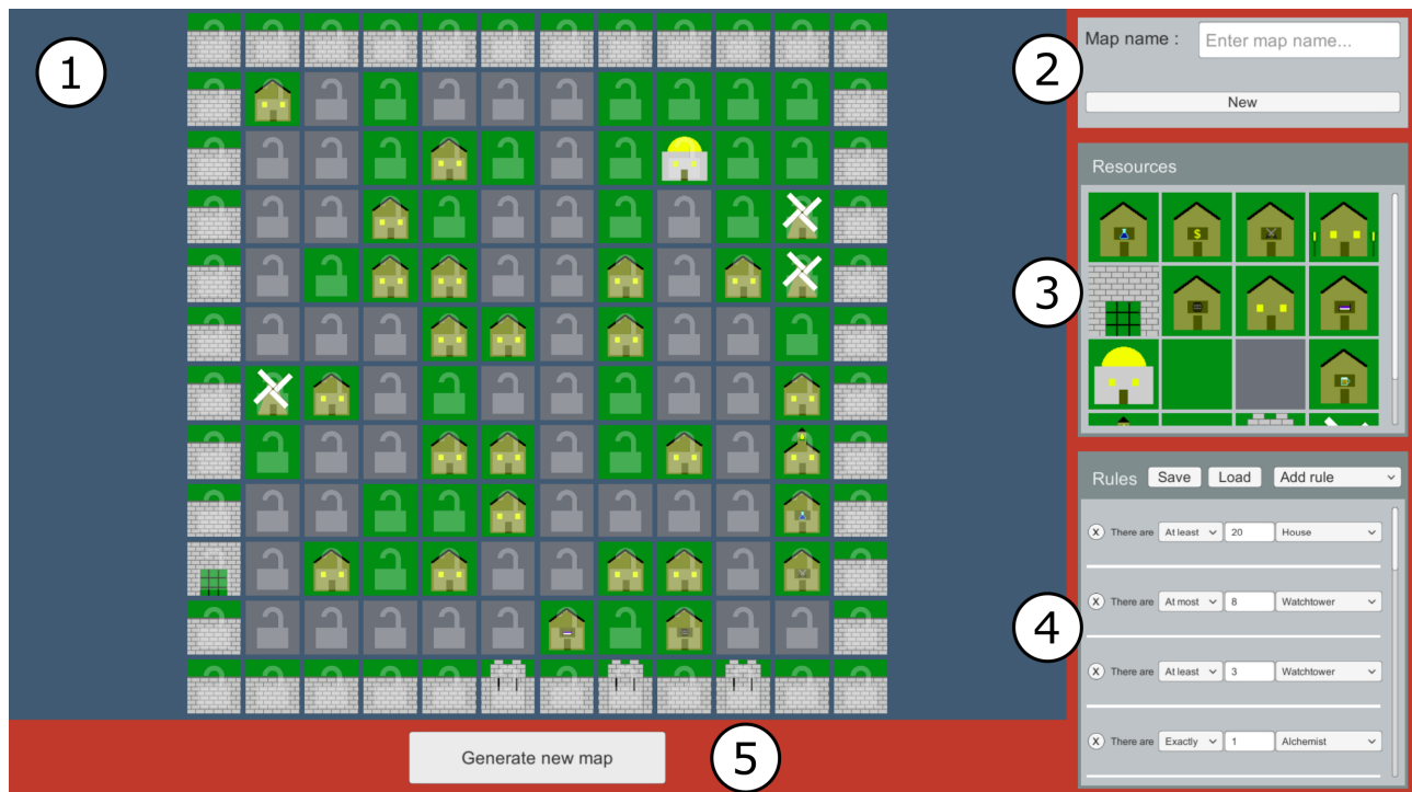
Figure 1: The tool's interface, with five distinct areas: (1) the interactive map, (2) a button for starting the creation of new maps, (3) the tiles available to the user and the map generator, (4) the rules that define the map generator, and (5) a button for generating new maps or re-generating the unlocked portions of the current map.
