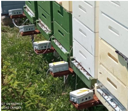
Figure 2: Installation of our hardware in the beehives at the Farkas méhészet apiary in Biatorbágy, Hungary. The waterproof boxes, containing a camera and a Raspberry PI, were bought at the electric hardware store. They are located in the front of the hive due to the camera capturing of the entrance and, also, due to ergonomics reasons (the beekeeper used to inspect the hives from behind, thus, the boxes are not in the way). The central unit containing a 4G WiFi router is located in a plastic box below the middle hive to which the sensors are connected by wires, the data processing unit is connected by WiFi. (We expect the sensors to break down in 2–3 years due to the conditions they are located in such that UV radiation, heat, frost, etc.)
