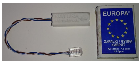
Figure 3: Audio sensor used in our project and its protection made on a 3D printer, both developed and manufactured by our project partner, the Natura mérnökiroda Ltd. A box of matches on the right is for showing the size of the hardware.
