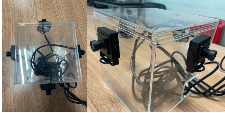
Figure 9: Four-directional camera: top view (left) side view (right)
