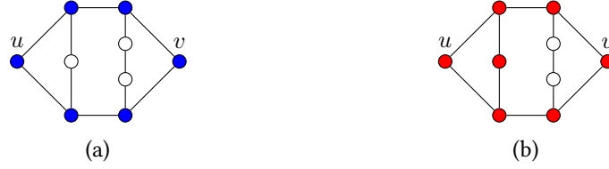
Figure 2: This figure shows (a) the geodesic interval [u, v] , i.e., the nodes on all shortest paths between u, v (blue) and (b) the geodesic closure \rho(\{u, v\}) , i.e., the smallest set of nodes that contains u, v and all nodes on all shortest paths between arbitrary node pairs of the set (red).
