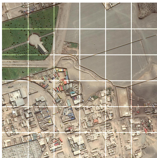
Figure 3: 1496 × 1496 image divided into 36 patches (256 × 256 pixels) with an overlapping region of 8 × 256 pixels between two patches.
