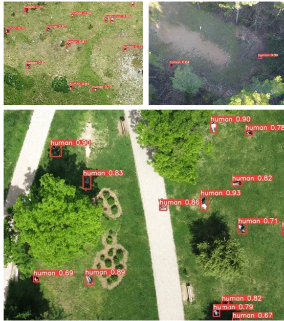
Figure 2: Examples of human detection on the HERIDAL dataset. Especially in this dataset, we have high-altitude scenes where it is sometimes difficult to detect people, even with the naked eye. In contrast, the computer vision model has proven effective in this difficult task.
