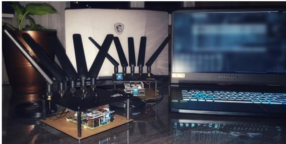
Figure 11: Raspberry Pis, with GPS and 5G Modules
