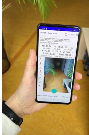
Figure 2: A user collects data using a smartphone, where magnetic field values are captured and stored together with the corresponding camera image. The current position at a predefined checkpoint is labeled by pressing a designated button.
