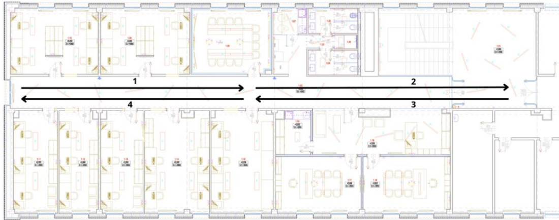
Figure 4: Floor plan with four classes for classification based on magnetic field values. Each class is defined by a corridor segment and a walk direction. Every segment is approximately 17 meters long.
