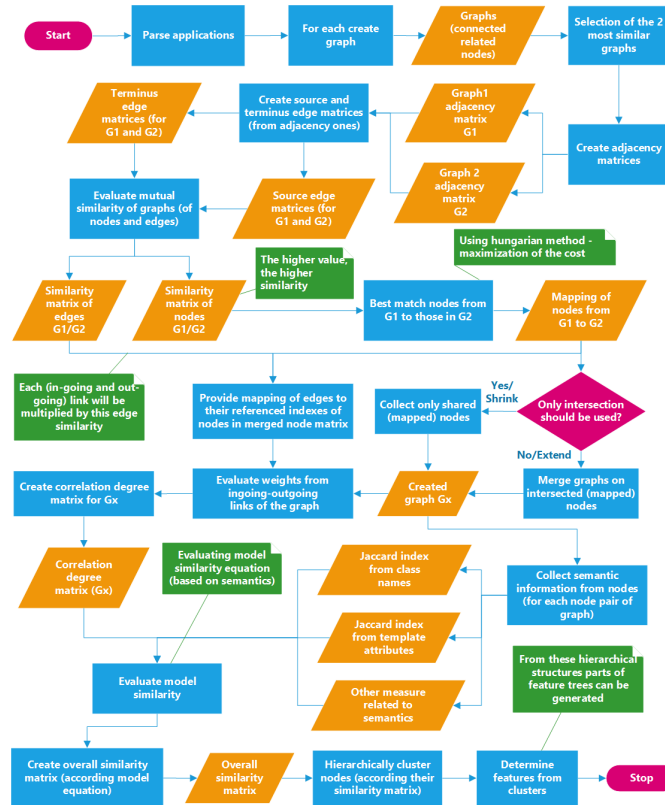
Figure 4: Matrix based structural/semantic analysis of features enhanced about node scores. Sources of integrated algorithms: [10, 15, 16].
