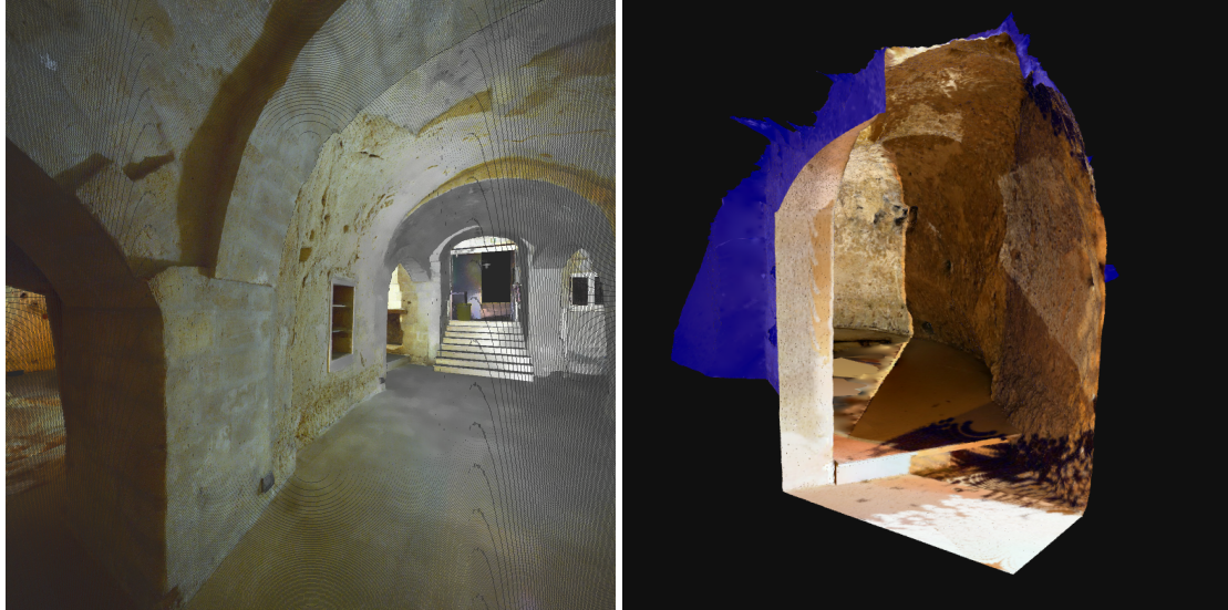
(a) An example of “LSP” file visualization representing one of the 6 views of a single TLS scan. (b) A visible fragment of 3D reconstruction of about 5.9M of polygons.
