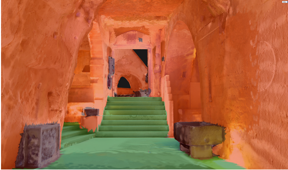
Figure 7: A view of the PC classification obtained with AI Classify function and manual correction in RC: red indicates walls and ceilings excavated or built with calcarenite, green represents flooring and stairs made of different materials, and purple identifies non-structural objects.
