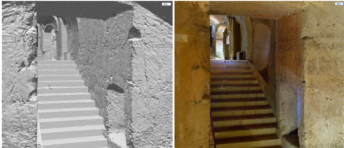
(a) Details of a 3D model fragment of a simplified reconstruction at 3M. (b) A reprojected textured 3D model fragment. The resolution of the whole texture is 16384 \times 16384
