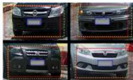
Fig. 7. Bounding box around the License Plate using Non-Max Suppression (NMS)
