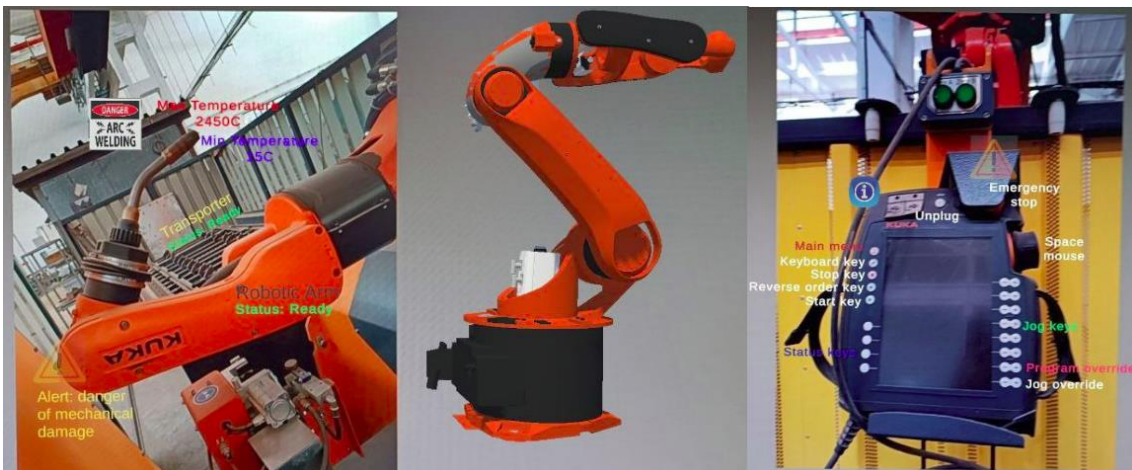
Figure 4: Window of the mobile application with the superimposed AR objects, messages and alerts.
