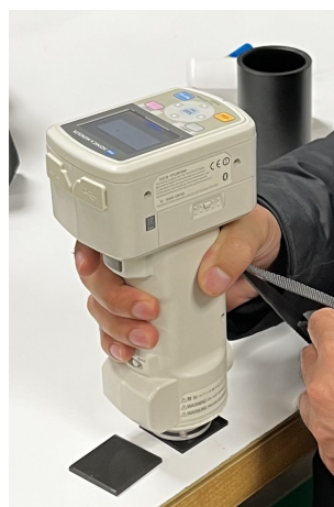
(d) Measuring L^*a^*b^* values of both surfaces.
