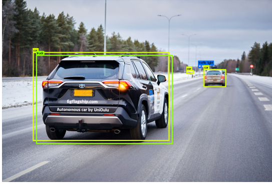
Figure 4: Recognized objects detected by the ready-to-serve object recognition service in the cloud/edge. 4
