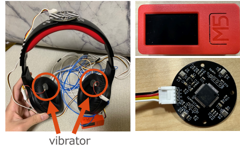
Figure 3: Headphone-type device (left), appearance (top right), microcontroller (bottom right), and microphone array
