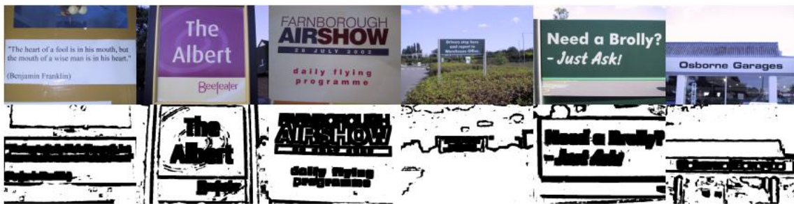
Figure 3 Text detection results: original images (row 1) and classification results (row 2). Neural classifier (6 inputs, 20 hidden cells and 2 outputs) using window size 17x17.
