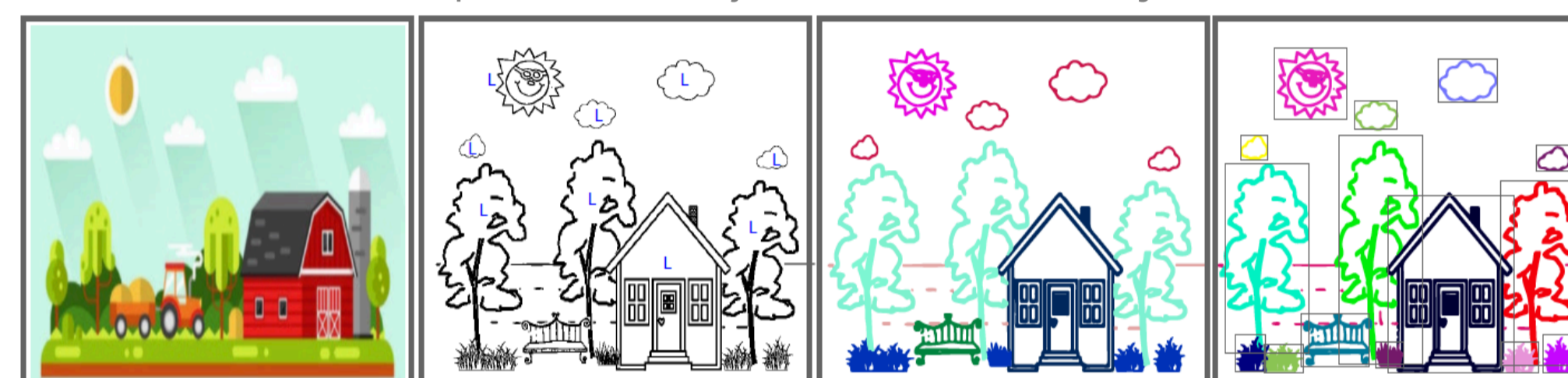
B. From left to right: reference image, synthesized scene sketch, ground-truth of semantic and instance segmentation.
