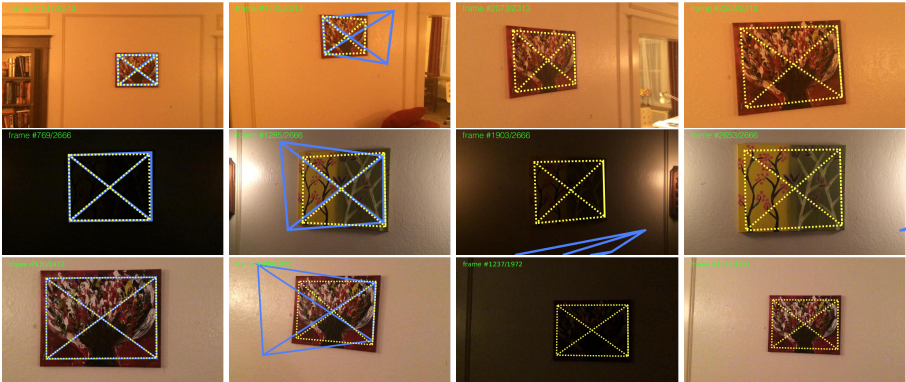
Fig. 10. Snapshots of tracking results. Blue: IC-LK; yellow: Conditional LK. The second image of each row shows where IC-LK fails but Conditional LK still holds.
