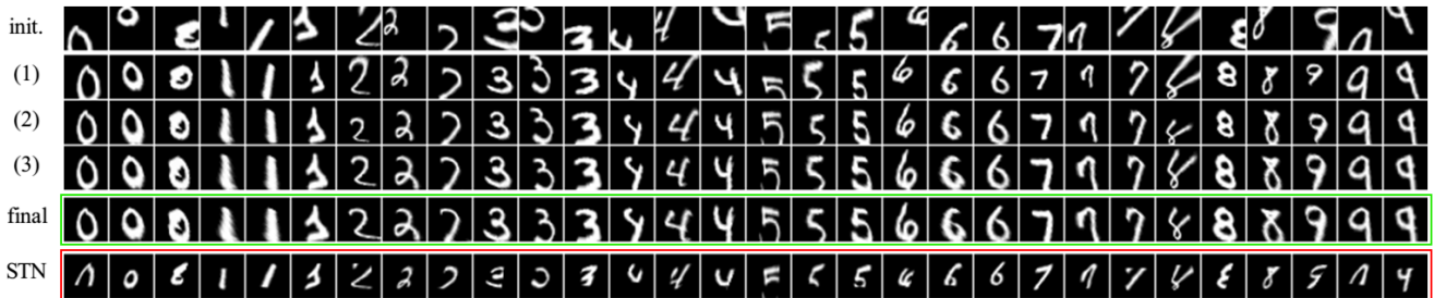
Figure 8: Sample alignment results of IC-STN-4(a) on the MNIST test set with homography warp perturbations. The first row of each column shows the initial perturbation; the middle three rows illustrates the alignment process (iterations 1 to 3); the second last row shows the final alignment before feeding into the classification network. The last row shows the alignment from the original STN: the cropped digits are the results of the boundary effect.
