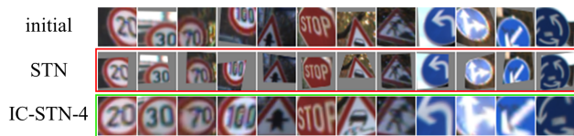
Figure 10: Sample alignment results of IC-STN-4 on the GTSRB test set in comparison to the original STN.
